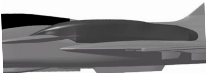
2 The dorsal conformal tank concept, low-speed proposal.
